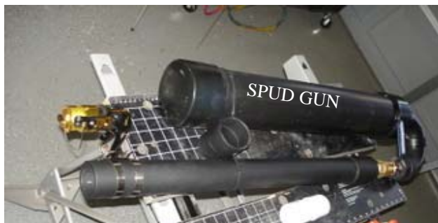
'SPUD GUN' Antenna Launcher Constructed by club President Ric Maxfield,
